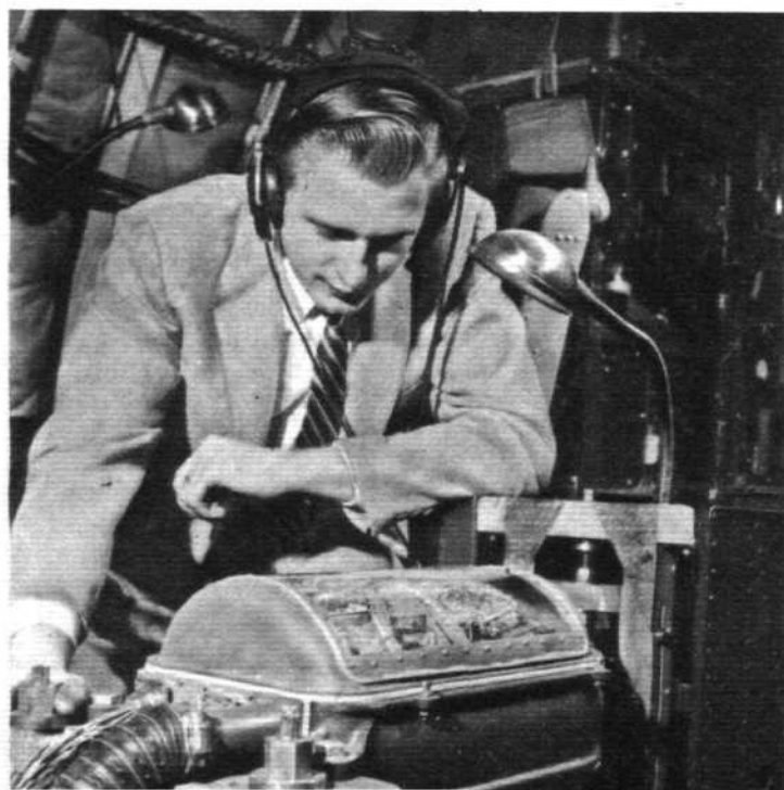
A stable platform for the Sperry inertial system for the B-58 Hustler being tested in a transport aircraft
