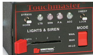
The Unitrol slide switch provides a tactile, long lasting way to control lighting and siren functions (available on most models).
